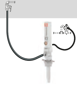
HOSE CONNECTION KIT 362 910 PM2 pump connection kit 1 m x 1/4" air hose 246 010, one 1/2" BSP (M) x 1/4" BSP (F) connection adaptor 945 516, 1 m x 1/2" oil hose with 1/2" BSP (MM) fittings, one automatic quick air coupling 1/4" BSP (F) 253 114 and one quick air connector 1/4" BSP (M).
