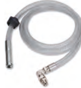
SUCTION ASSEMBLIES AND SUCTION HOSES Suction assemblies for wall mounted stub pumps. Assemblies include Ø 42 suction tube with foot valve, height adjustable 2" bung adaptor and 2 m x 3/4" rubber connection hose.
