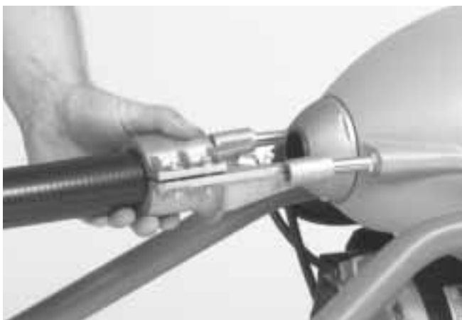
Figure 3 – Rear Guide Hose Attachment
