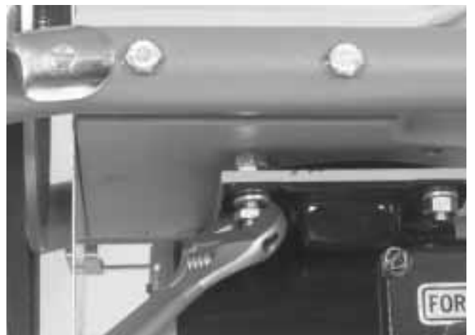
Figure 14 – Removing Clutch End Play
