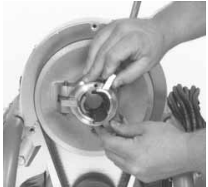
Figure 13 – Replacing Clutch Jaws
