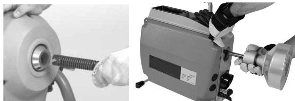
Figure 4 – Inserting Cable Into Front Of Machine
