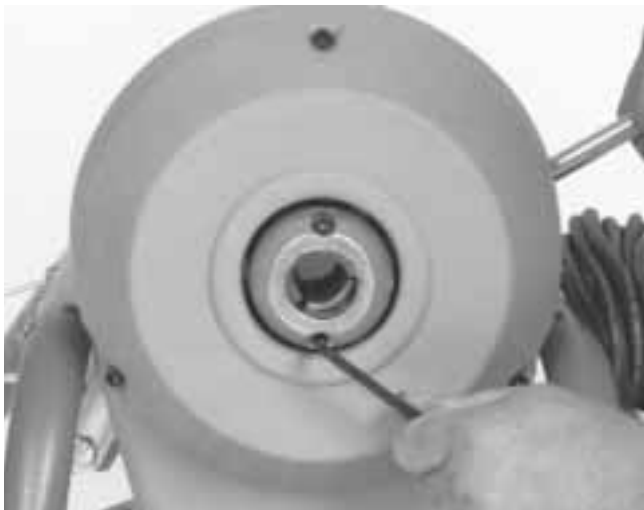
Figure 12 – Replacing Clutch Jaws
